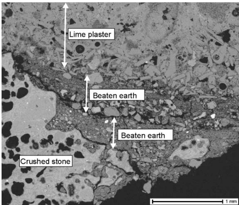
Figure 7 SEM image of the sample 669.
